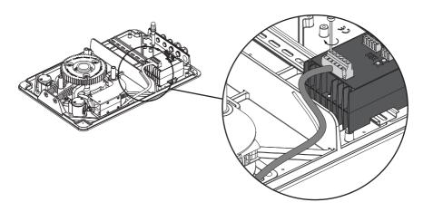
Plug in the cable and make sure to tighten all six screws. Make sure the numbers on the control
