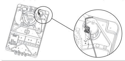
• Slide the counterclockwise module over the axis.
