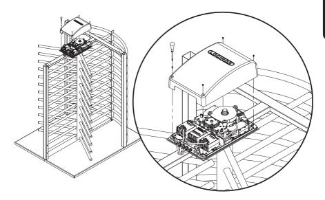
• Make sure the that the rib fits the corresponding groove in the cover
