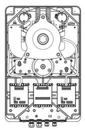
• Be sure the top chassis is mounted correctly before screwing it down.
