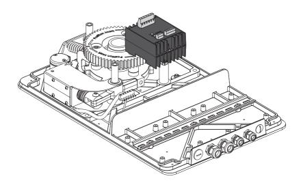
Connect the clockwise module with the control unit.
