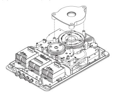
• Check the concentricity between the bearing and the blocking disk (Due to spring tension, the allignment of these 2 components can differ)
