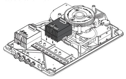
• Connect the clockwise module with the electrical control unit & tighten the screws
