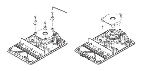
• Remove the spacing tubes: The base mechanism is now ready for optional modules
