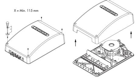
• Loosen the top chassis bolts, and remove them
