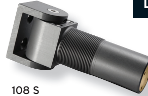
108 S Item#: 75108113 SELF-CLOSING FROM 85° • Holds gate open at 90° • With Final Snap Action
