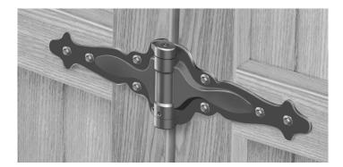
Hinge RANGE Maximum Self-Closina Weight Maximum Gate Dimensions **REGULAR RANGE** 55lb (25kg) per pair \*5'Hx3'W (1524x915mm) \*Always space the hinges as far apart from each other as possible for maximum holding strength.
